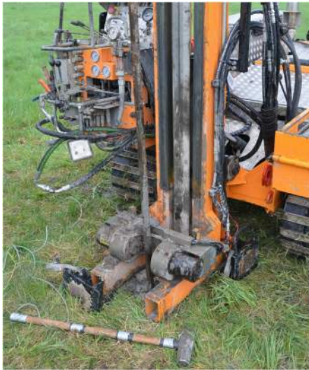
Fig. 4. Seismic cone penetration test equipment with two pre-loaded L-shaped plates, SCPT probe and a sledge hammer connected to the DAQ to trigger recording.
